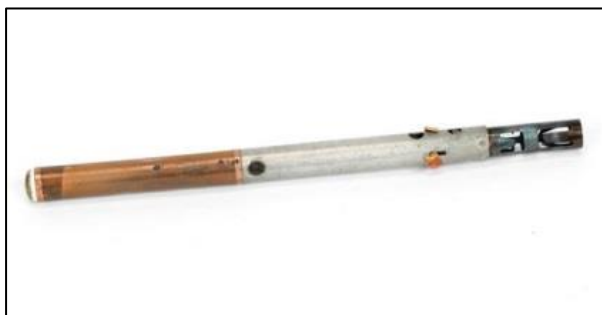
Figure 38: Pencil Time Fuze Within this fuze, a striker was held back by a steel wire kept under tension. Once a glass ampoule was broken, a corroding solution was brought into contact with the wire. When the wire broke, the striker was released and operated a percussion cap attached to a short Bickford fuse. 7
