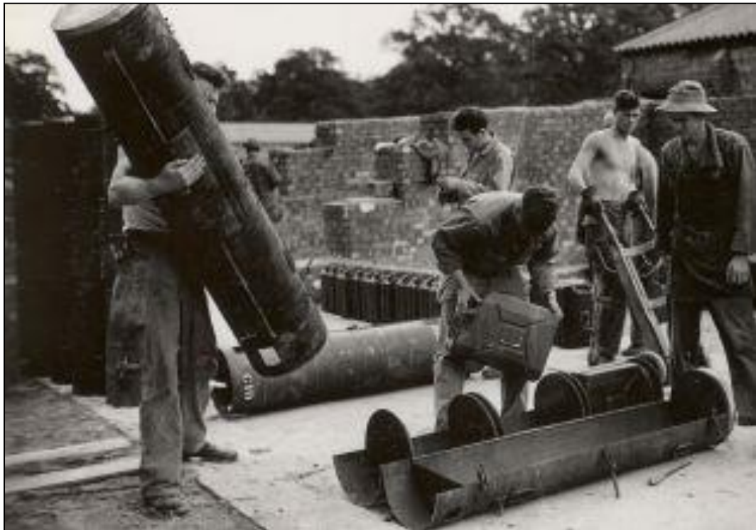
Figure 75: The Type 'C' container, as shown at the Office of Strategic Service's (OSS) packing facility at Holmewood, was of a cylindrical shape formed from reinforced sheet metal. Split into two, the container was secured with three latches which once unlocked allowed it to open fully along its length. 80
