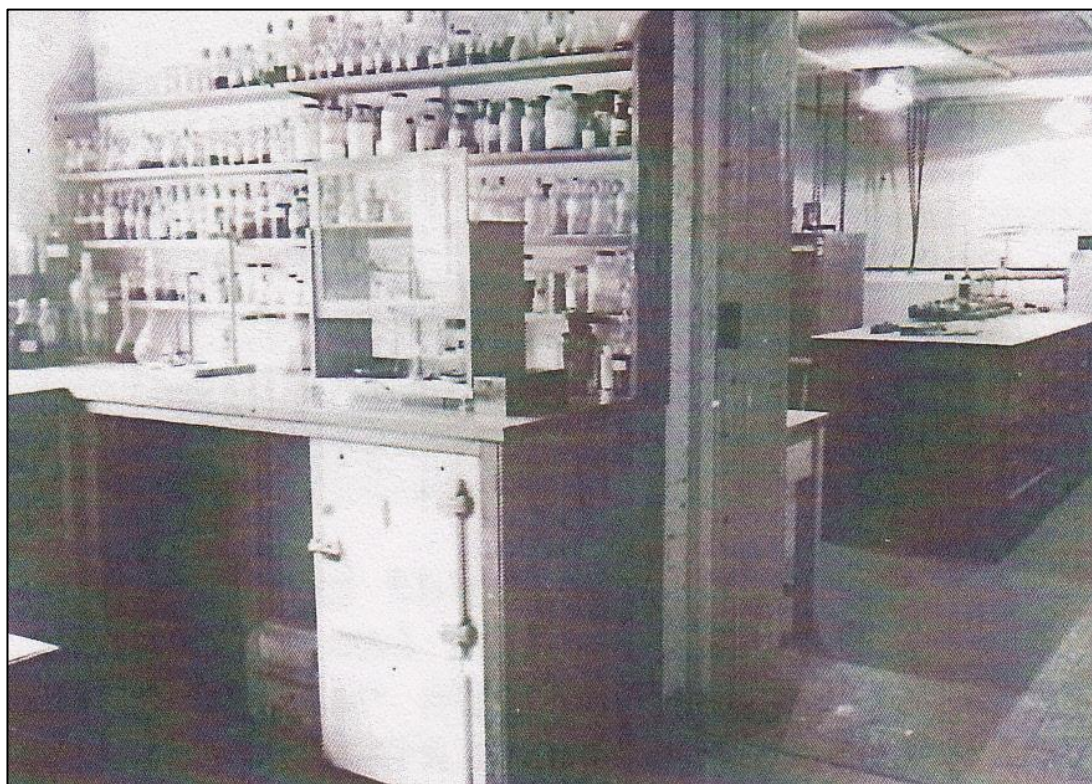
Figure 46: Interior of the ThermoStat Hut. The room in the foreground is the analytical and plating laboratory, in the background, the thermostat room. The laboratory was well equipped with standard equipment which included a physical balance, jigs, soldering and glassblowing equipment, inorganic reagents together with specially prepared inorganic solutions, organic solvents, fume cupboards, a Gallenkemp Oven, a smaller oven and a refrigerator. 47
